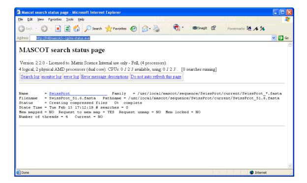
If an error occurs, use the links to the monitor log and the error log to investigate the cause. If all is well, you will see the following messages displayed on the status line for SwissProt:
