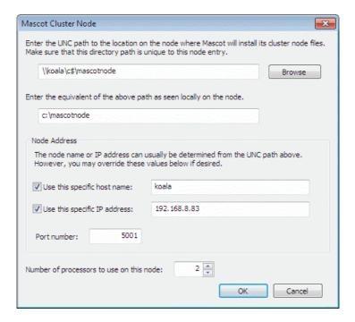
Use the Browse button to ensure that the UNC path to the node is correct. If the machines are in a Windows domain, and the remote drive is not explicitly shared, you can enter C\$ for drive C, etc., to use the administrative shares. If the base directory does not exist, create it using the 'Make New Folder' button. The recommended base folder name is MascotNode.
