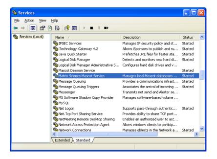
Highlight the entry for Matrix Science Monitor Service and press Start. If the service fails to start, the cause must be investigated and the problem fixed before proceeding.
