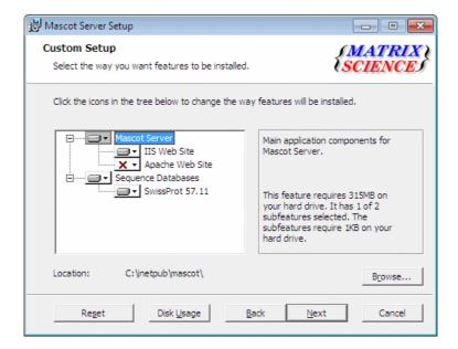
If IIS is installed and functional, the default choices are as shown above, with IIS being configured automatically. If you don't have IIS installed, the Apache option will be selected instead. A test for whether Apache or some other web server is actually installed comes later.
