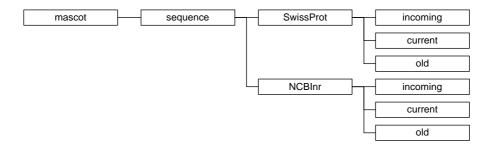
For each database, the *incoming* directory provides a workspace for downloading and expanding a new database file. The *current* directory contains the active database, and this is where Mascot Monitor creates the memory mapped compressed files. The *old* directory is where the immediate past database file is archived ... just in case.
